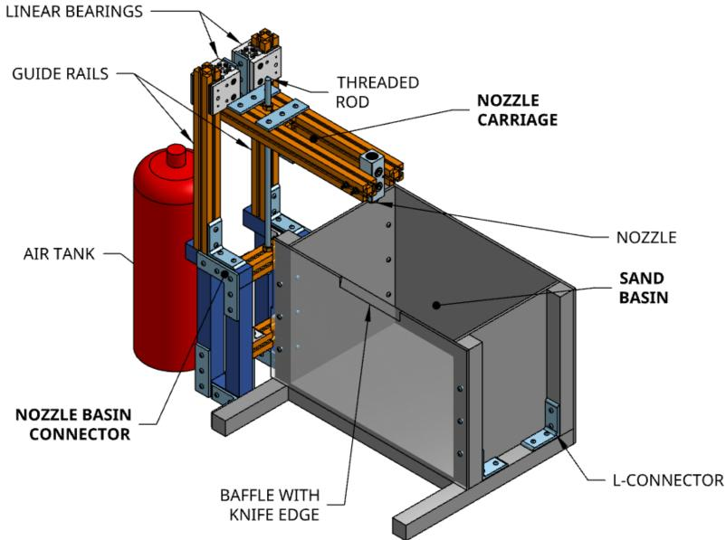
The team conceptualized an apparatus featuring a clear baffle with a knife edge to separate the jet flow. The rig structure works as an extended beam from the tank for the flow to impact on the surface, as well as a threaded rod for height adjustment. Images of the half-crater formed will be captured to measure its depth and width. The experiment will be performed by maintaining the nozzle's relative elevation, or height divided by diameter, constant throughout the experiment.
